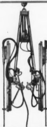
★ The SDR 34 shaft sinker for faster shaft sinking. Fully closed it's 5'6" between drill centers; open 19'3". All adjustments quickly made with air motor.
